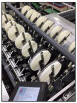
Suntreat purchased two of Hurst's patented Dual Cassette Systems, which allows it to run four different style PLUs at the same time. This configuration gives the company the advantage and flexibility to label with all 12 labels while only using two banks and still utilize all their drops and pack bins.
